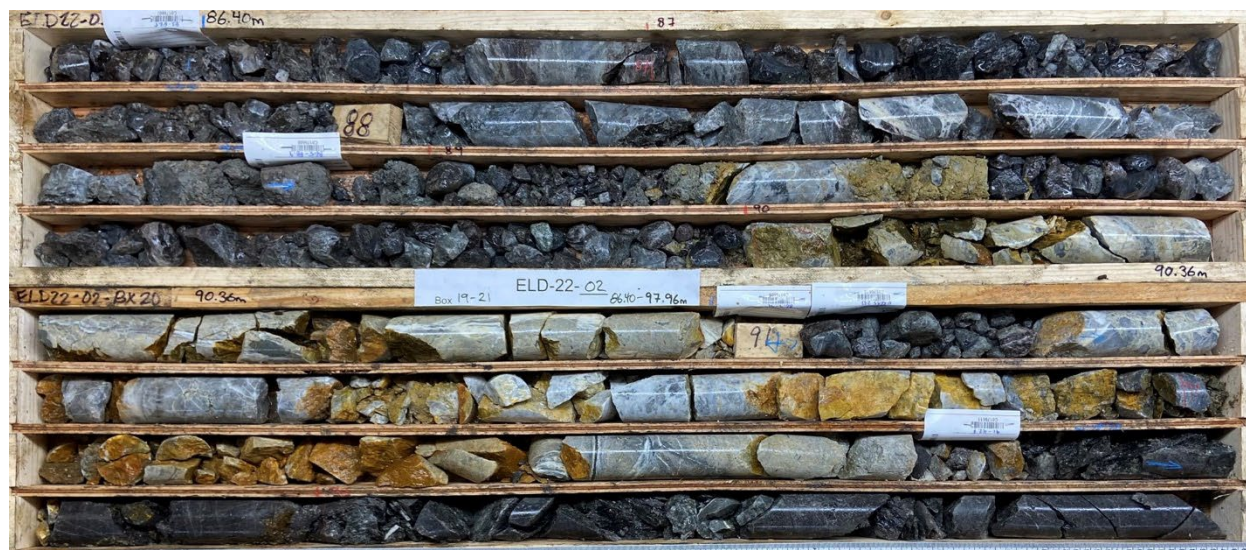
Figure 4: ELD22-02 core from 86.4m to 94.3m, showing silicified breccia and veining.
