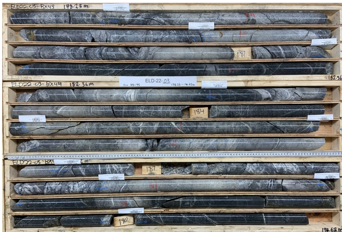
Figure 5: ELD22-03 core from 178m to 193m, showing diorite cut by several quartz-carbonate-sulphide veins and vein breccias.
