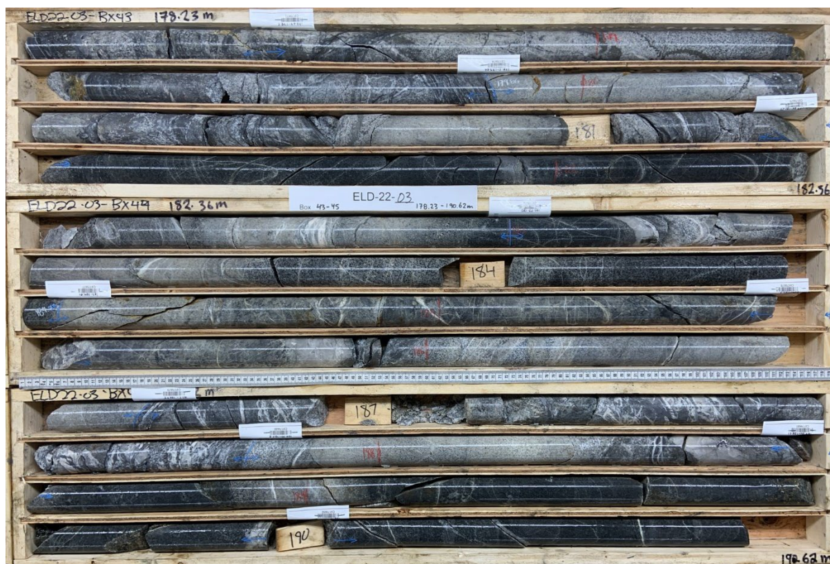
Figure 6: ELD22-03 core from 178m to 193m, showing widespread argillic alteration of diorite cut by numerous, close-spaced quartz-ankerite-sulphide veins and vein breccias. The lower box, from 186.8 – 187.8, returned 1.05m at 3.11 g/t Au.
