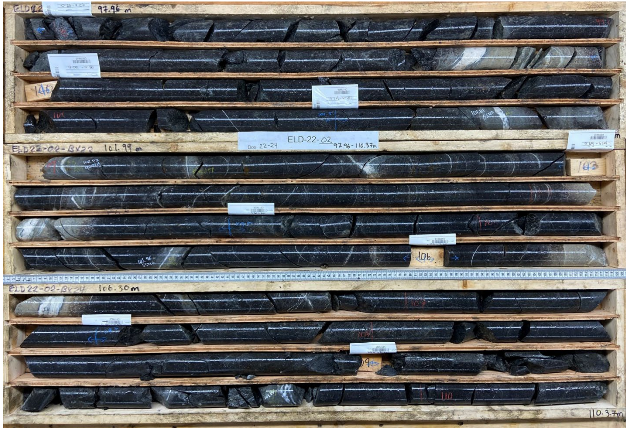
Figure 4: ELD22-02 core from 98m to 110.4m, with several narrow quartz-sulphide breccias and veins. The interval from 109 – 110.5m returned 0.511g/t Au.
